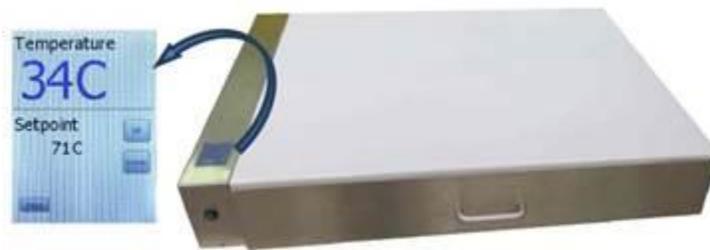
1. Turn on power to the Dry Heat Convection Oven by using the main switch on the side.
